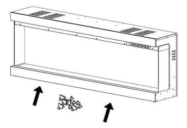
**4.** After placing the fuel bed media, fasten screws back on the glass panel.
