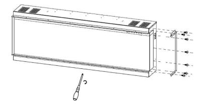
4. Remove the screws from the fireplace as shown in the picture below.
