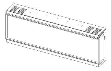
2. Remove the 7 screws on the left side. Take off the fending bar and panel.
